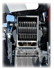
Thanks to the well-balanced material distribution and the effective fitting of the hammers, milling performances of up to 25 tonnes of grain per hour are not uncommon.
